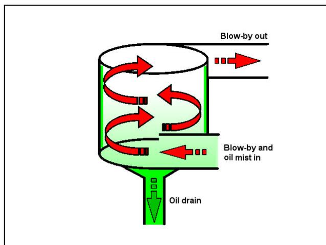
Figure 11: A simple non-driven centrifugal oil separator.
