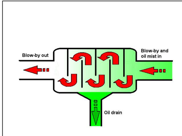
Figure 10: A simple labyrinth oil separator.
