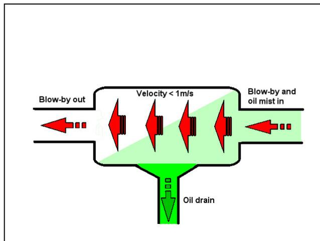
*Figure 9: A simple oil separator volume.*
