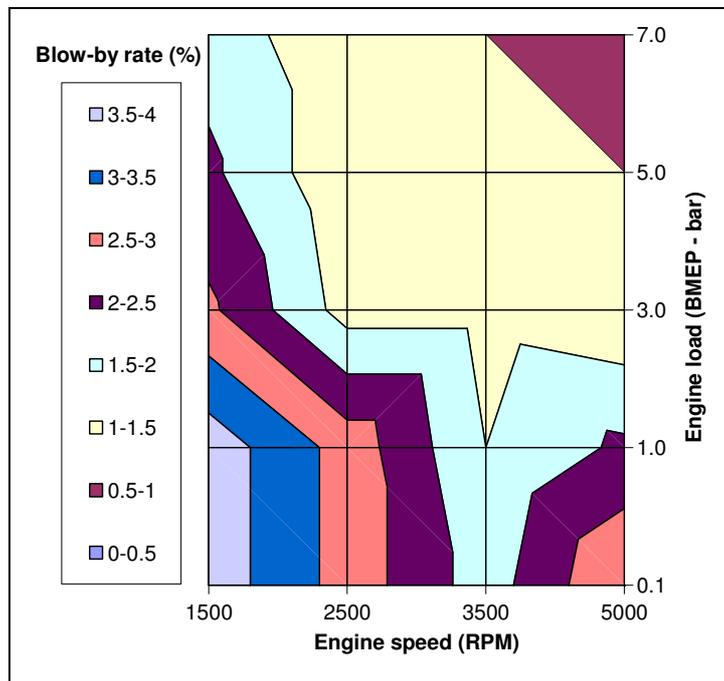
Figure 2: Blow-by rate map for a normally aspirated 1.6 litre gasoline engine [1].
