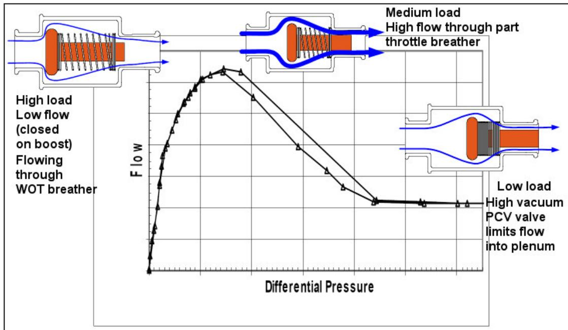
Figure 7: Typical PCV valve flow versus pressure [3].
