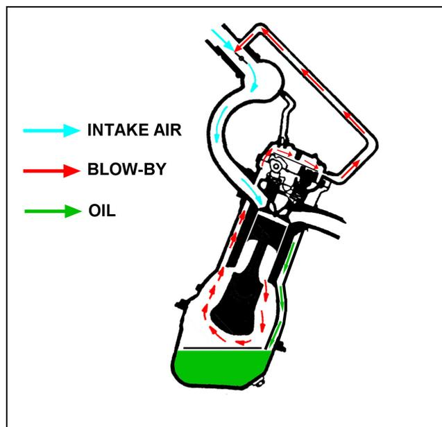
*Figure 6: High blow-by / high load breather flow.*
