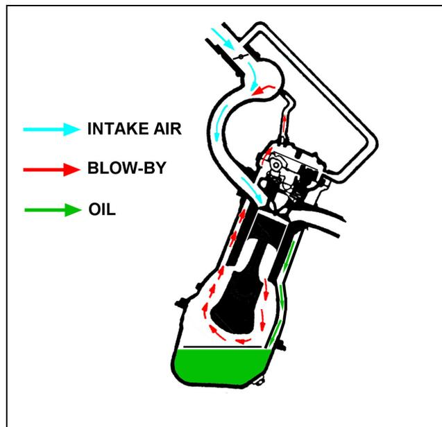
*Figure 5: High blow-by / low load breather flow.*
