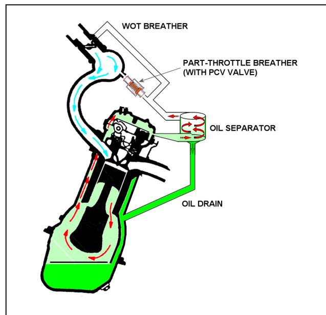
Figure 12: An external oil separator.
